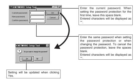
The following Password Request screen will appear for VN-C2U set with password protection. VN-C2U setup cannot be made unless the password matches.
